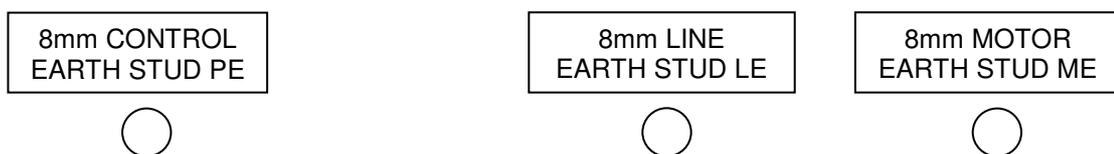
All control panels have various earth studs located near the various terminals, there is a dedicated stud for the line and motor earths. All earths to the external equipment should go to the control earth stud below the terminal rail.
